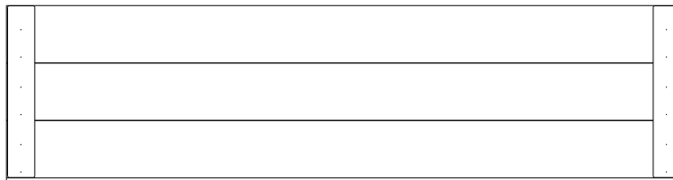
RP6 | ROOF PANEL - W2A02627 (4) | 1 5/8"x15 5/8"x59" (42x396x1499)
