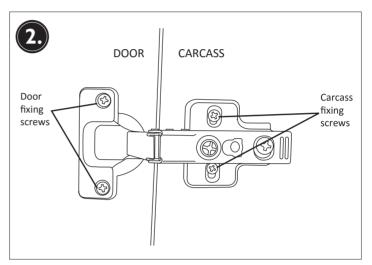
Choose the desired handing and fix hinges to the door and then the carcass. Holes are also provided on both ends of the door for the badge attachment to be fitted once the desired handing is chosen.
