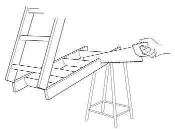
Saw off the excess piece of the ladder on both sides.
