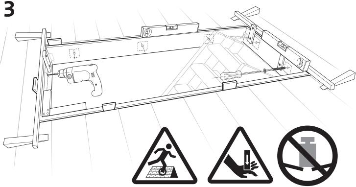
Use a set square on each corner to guarantee a 90° angle. Where necessary use packers (not supplied) to fill the space between the frame and joists. Use a spirit level on all horizontal plains to ensure the frame is level. Finally drilling through part No. 1 and into the joists, make ten 6mm holes at intervals shown in the diagram. Then use the wood screws (not supplied) to affix the frame into position.
