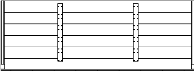
RP1 | ROOF PANEL - W2A03279 (x2) | 1 3/4"x19 1/4"x53 3/4" (45x490x1366)
