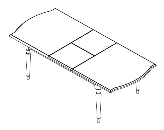
**IMPORTANT:** WHEN LIFTING OR MOVING THE TABLE ALWAYS DO SO FROM THE UNDER FRAME AND NOT THE TABLE TOP
