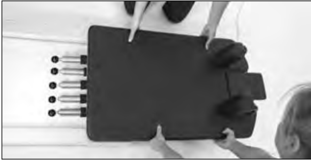
5. Slide rollers into c-channels.
