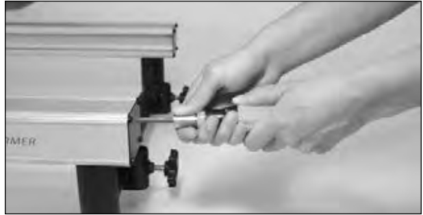
2. Using a Phillips screwdriver, remove stopper plates.
