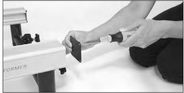
6. Using a Phillips screwdriver, replace stopper plates.
