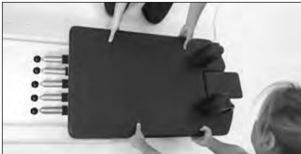
3. Carefully slide carriage out of the aluminum rails keeping carriage level until completely free of rails. Turn carriage over ensuring rollers are secure and do not come in contact with the floor.
