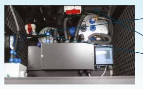
Open the vent and you can change the filter and open/close ball valves inside.
