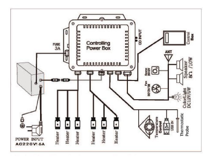
Connect the wires at the rear of the shower, pairing the corresponding labels.
