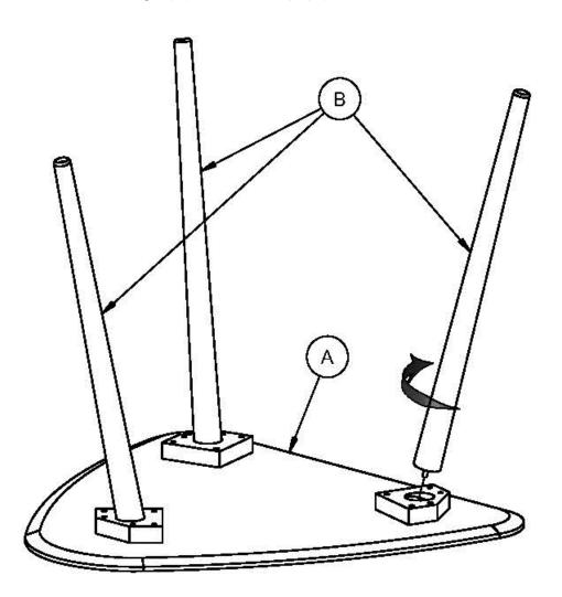
**IMPORTANT:** To avoid damage to the parts, tighten fixings by hand only. We would advise that at this stage the top remains inside the original packaging, or lay onto a clean carpet or banket to avoid damage to the surface.
